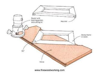
When building a large picture frame for a friend, I needed to add keys to the miters for strength. The problem was that the frame was more than 60 in. long on each side. In the past, I had always used a simple cradle jig on the tablesaw to hold the frame upright while cutting the slot. But this frame was much too large for that. My solution was to use this simple fixture and a bottom-bearing-guided, slot-cutting bit in a router.
